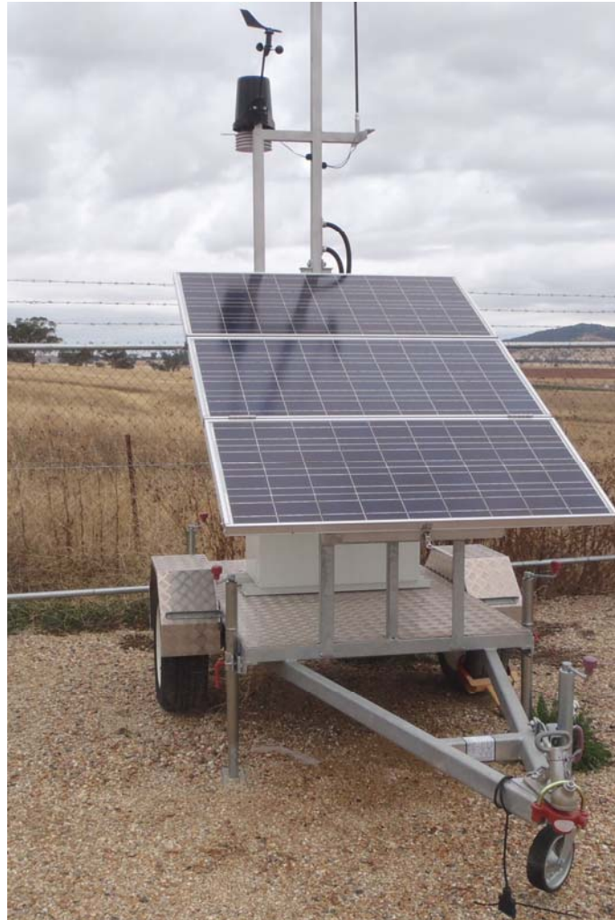
Figure 11 Continuous noise monitoring trailer with WCC mine in background
