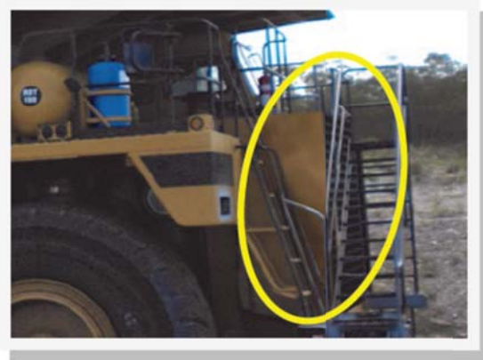
Figure 8: Example 785 Acoustic Enclosure on the Radiator (from Humex, 2012)
